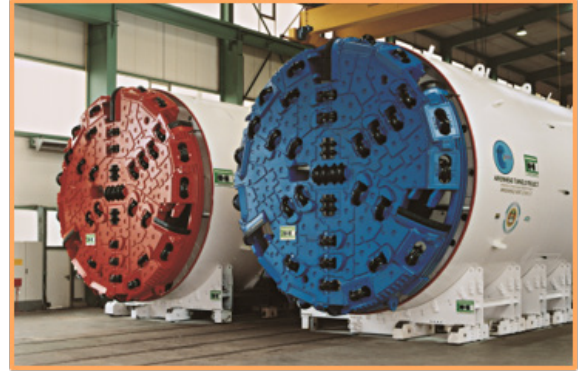
Arrowhead Tunnels Boring Machine
