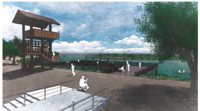
2 Perspective 2 : This perspective is the view from the levee on Bethel Island looking towards the fishing dock and the observation tower. There are two stairs to get on the levee and one stair attaches ADA ramp. The fishing dock has a pavillion, fish cleaning stations, trash cans, and benches. The observation tower has 3 stories and a height of 38 feet.
