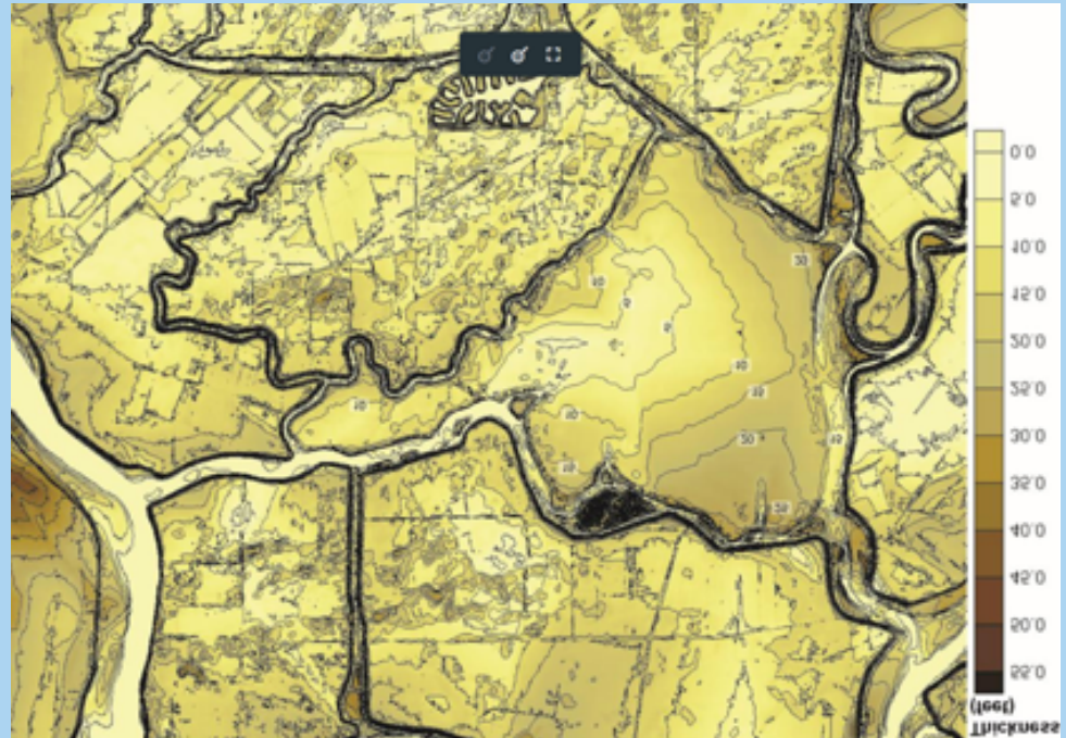
Peat Thickness. Average peat layer thicknesses across Franks Tract. The data derives from borings within Franks Tract (HLA 1990), from adjoining islands and tracts (USGS 1982), and Jersey Island and Bouldin Island quadrangle sheets. The data suggests that the deepest peat deposits exist around the northeast extent of Franks Tract, with layer thicknesses of around 25 feet deep. Going east to west, the thickness of the peat deposits decreases gradually to around 10 feet deep in the center of Franks Tract, down to less than five feet at the transition to Little Franks Tract. By comparison, peat deposits on Sherman Island on the west side of the San Joaquin River are as much as 55 feet deep. Source: Moffat & Nichol 2017.
