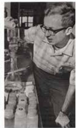
GAYLON RODIN FILTERS A SAMPLE. He's checking for presence of bacteria.
