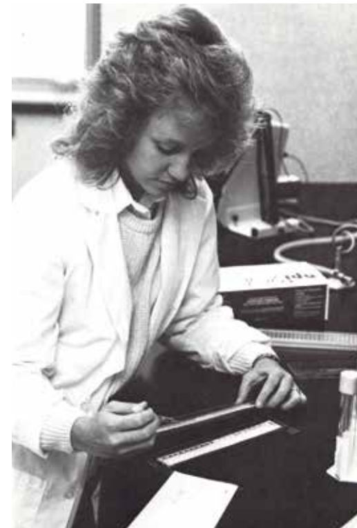
MWD CHEMIST LOUIS GIMAN RUNS WATER HARDNESS TEST IN LAB. Paul Evans, chemist, (background) checks sample for manganese content.
